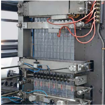
Draw - off rollers for pulling film and vertical sealers
