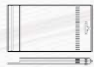
Side Seal Bag with Sheet insert, Ultrasonic Header Seal and Euro punch
